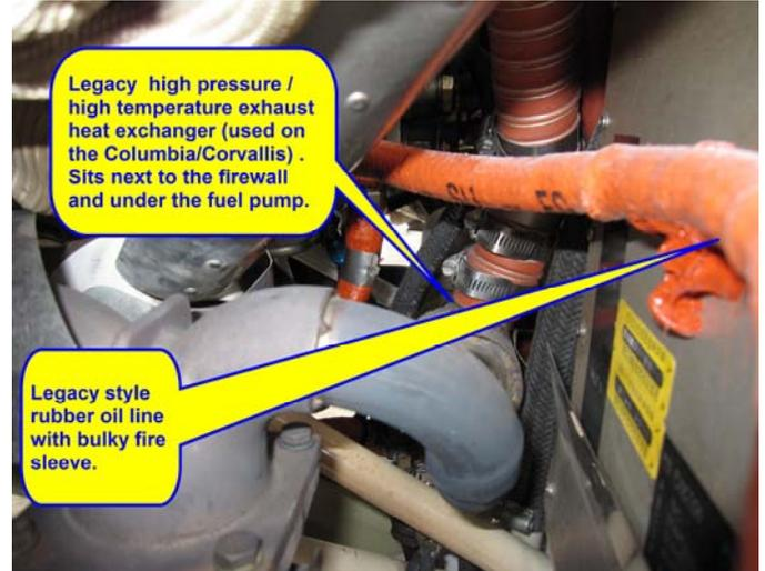
Legacy high pressure / high temperature exhaust heat exchanger (used on the Columbia/Corvallis) . Sits next to the firewall and under the fuel pump.
