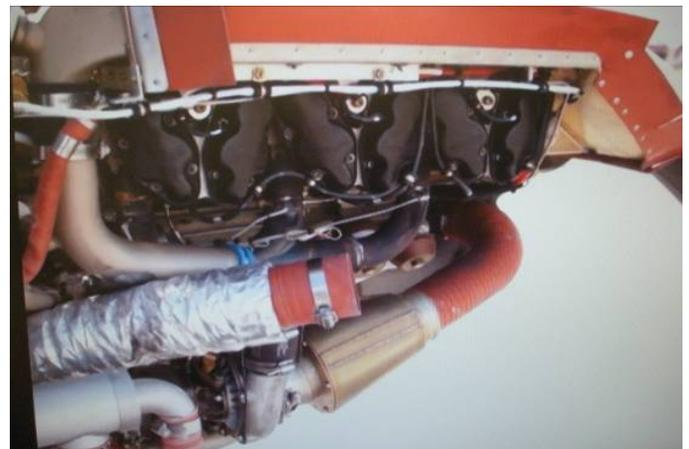
There is no effort to install heat shields around the turbo section, even though it often operates near 1700 degrees F on the TCM system installed in the SR22T.
