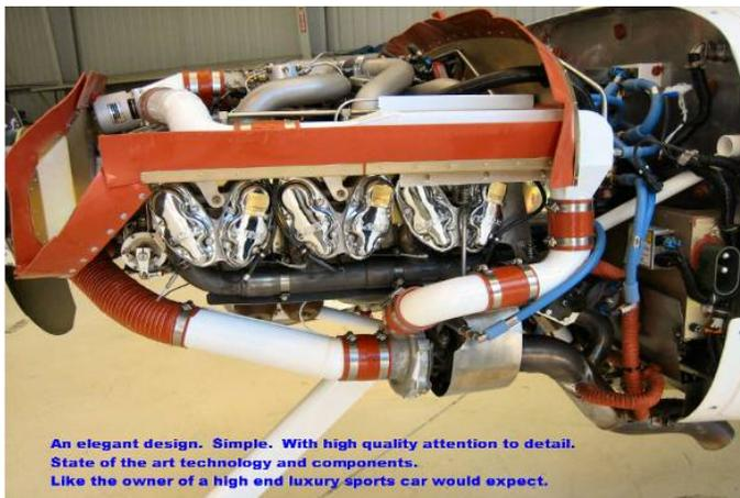
Note the blue silicon high temperature "lifetime" oil lines and the stainless steel heat shield around the hot section of the turbo charger.
