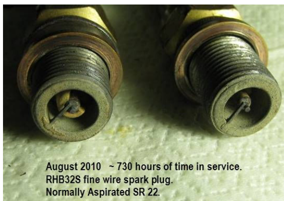
Figure 1. An example of two cracked fine wire RHB32S spark plugs from one engine.
