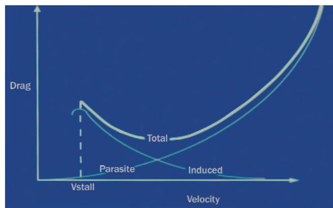
Figure 2: Indicated airspeed vs drag.
