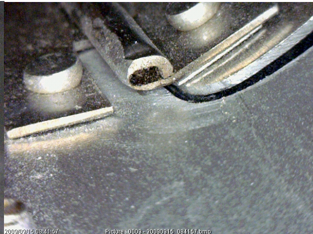
Crimped hinge pin retention
