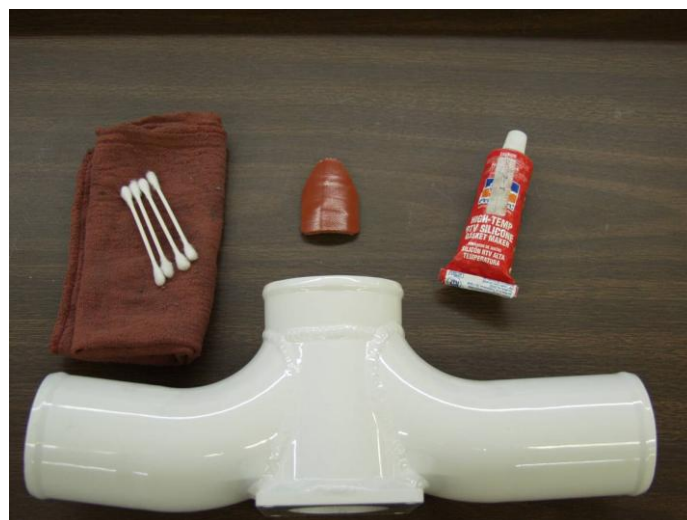
Figure 2 shows all material needed to attach the Anti-Wear Pad to the PRV/Y tube
