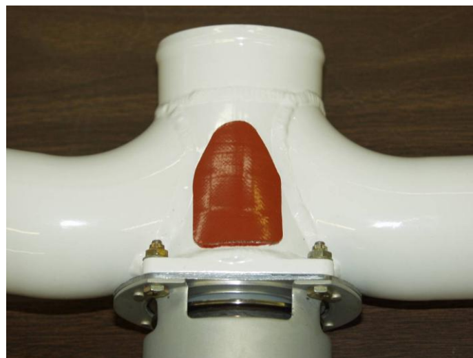
Figure 3 shows the Anti-Wear pad properly attached to the underside of the PRV/Y tube.
